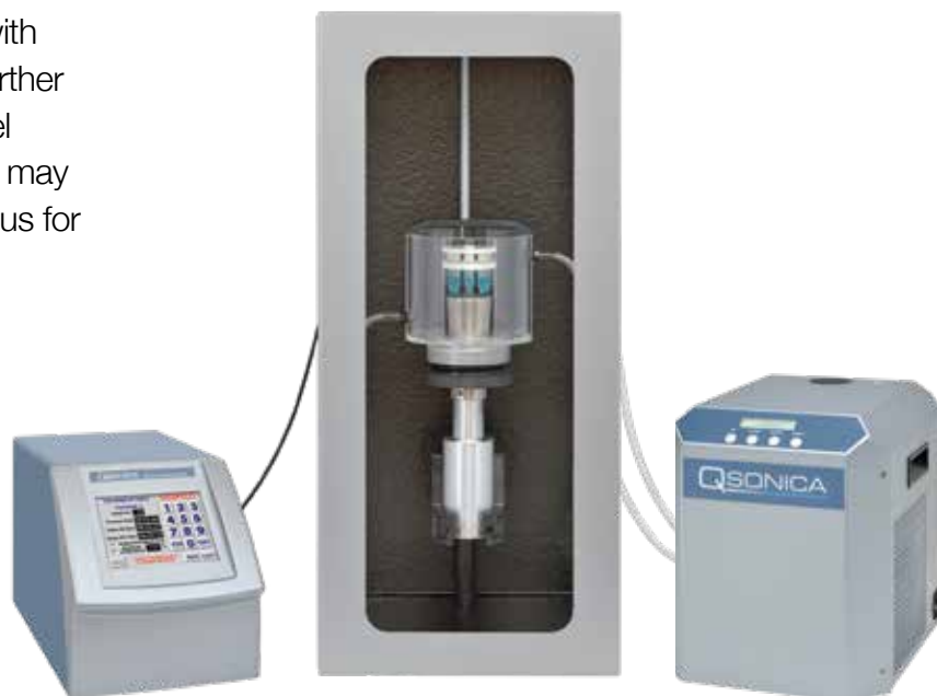
Chiller shown with Sonicator, tubing set, Cup Horn and Sound Enclosure (sold separately).
